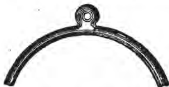
Fig. 34—Showing the Piece Ready for Rounding and Welding.
