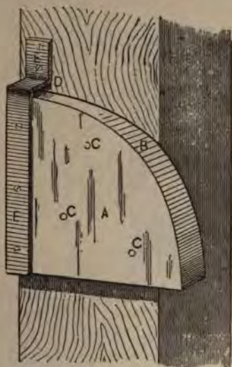
Fig. 69—A Cheap Tire Bender, as Made by "R. C."
