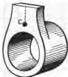
Fig. 28—Showing the Piece After the Rounding and Welding Operations.
