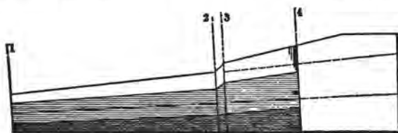
Fig. 146—Pattern for Laying Off Axles to Receive Thimble Skein.
