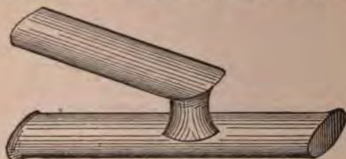
Fig. 141—Showing Finished Offset.
