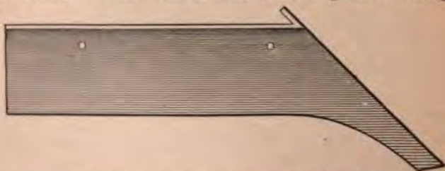
Fig. 342—Showing the Share Completed.
