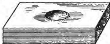
Fig. 87—Showing how the Block is cupped.
