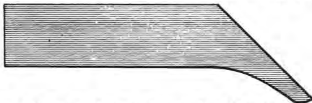
Making a Plowshare. Fig. 338—Showing how the Steel is Shaped at First.
