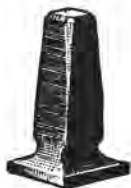
Fig. 3—Light Flatter for Finishing Flat Iron. Made of 1\frac{3}{4} square Steel. Face 2\frac{1}{2} inches square.
