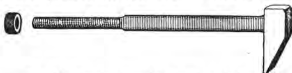
Fig. 66—Showing how the other Piece is forged.
