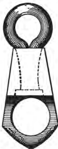
Fig. 288—Front View of the Swivel, Showing how the Tug is Opened Up.
