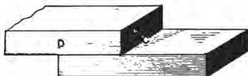
Fig. 76—Showing how the Pieces might be Lapped.
