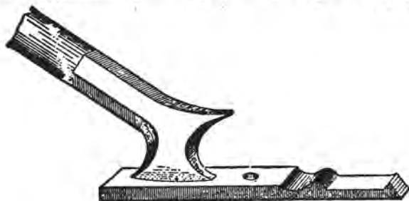
Fig. 140—Showing Finished Stay End.
