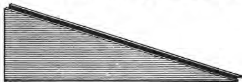
Fig. 28--Singletree Clip Wedge.
