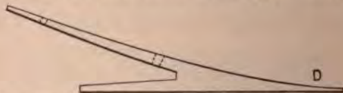
Fig. 350—Showing the Two Pieces of Steel seen in Fig. 349 Drawn to a Point.
