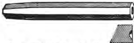
Fig. 34—Tool for Rounding Rivet Heads.
