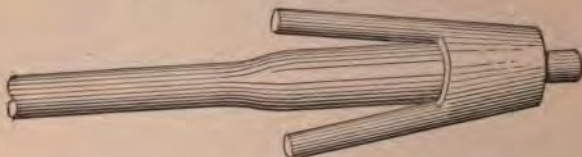
Fig. 278—Showing how the Ends are Turned.
