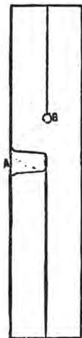
Forging a Dash Foot by "J. C. H." Fig. 197—Showing how the Iron is Fullered, Punched and Split.
