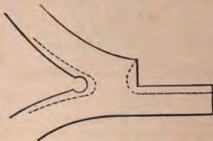
Fig. 136—Stay Offset Opened to Forge as in Dotted Lines.
