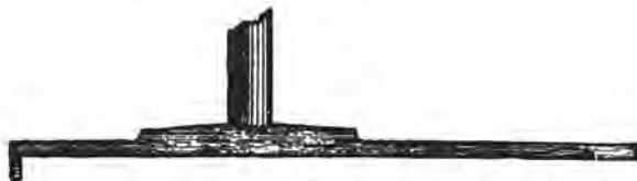
Making a Locomotive Valve Yoke by the Method of "R. D." Fig. 259 —Showing the Piece Ready for Bending.
