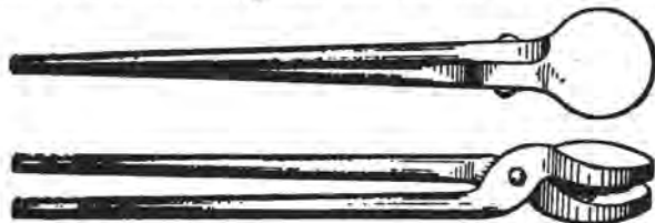
Fig. 12—Tongs for Holding Horseshoes.
