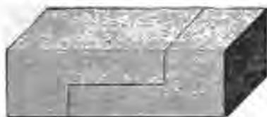
Fig. 222—Showing the Lines on which the Iron is Split
