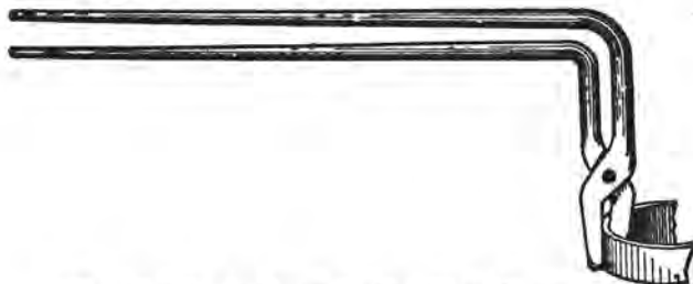
Fig. 16—Handy Tongs for Handling Wagon Tires.
