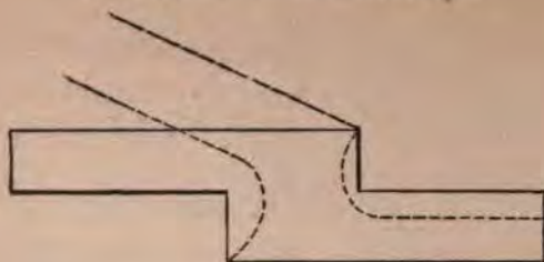
Fig. 134—Showing the Piece as Forged and Fullered.
