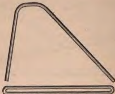
A Tool for holding Slip-Shear Plows in sharpening. Fig. 38—Showing how the two Pieces are shaped,
