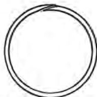
Fig. 126—Showing how the Ferrule is bent.
