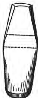
Fig. 68—Showing how the Chisel is Beveled.
