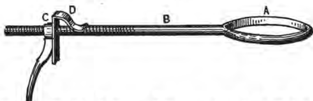
Fig. 181—Tool for Pulling on Felloes, made by Louis Tuthill.
