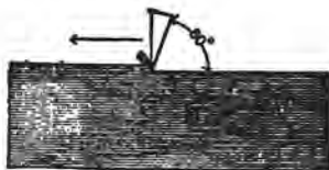
Fig. 62—Showing the Bottom Face at an Angle of 80 degrees to the Line of Motion.
