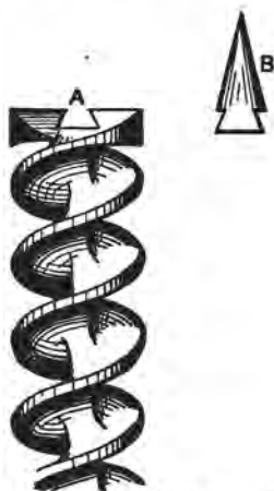
Fig. 196—Repairing an Auger. Showing Notch and Piece to be Fitted into it.
