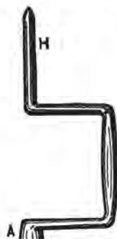
Fig. 82—A Home-Made Drill, showing How the Shank H is Formed and the End A Upset.
