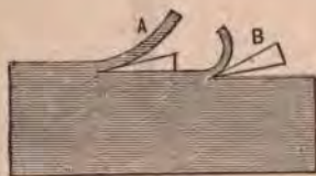
Fig. 61—Showing that the Effect of the Cutting Edge depends upon the Angle of the Bottom Face to the Chisel's line of motion.
