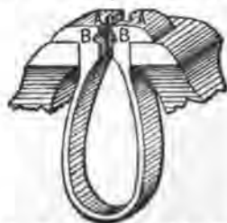
Fig. 162—Showing the Device adapted for Holding Round Pins. of the accompany engravings, and has a groove in its jaws to hold the round stems of bolts to the vise
