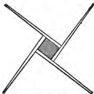
Fig. 123—Manner of Attaching the Fans to the Shaft of Blower.
