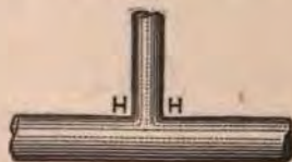
Fig. 116—Incorrect Way of Finishing.
