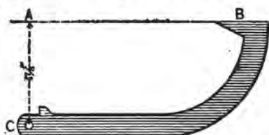
Fig. 185—Making a Cant-Hook. Showing Method of making Shoulder.
